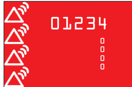
System fault alarm (red) with error code
